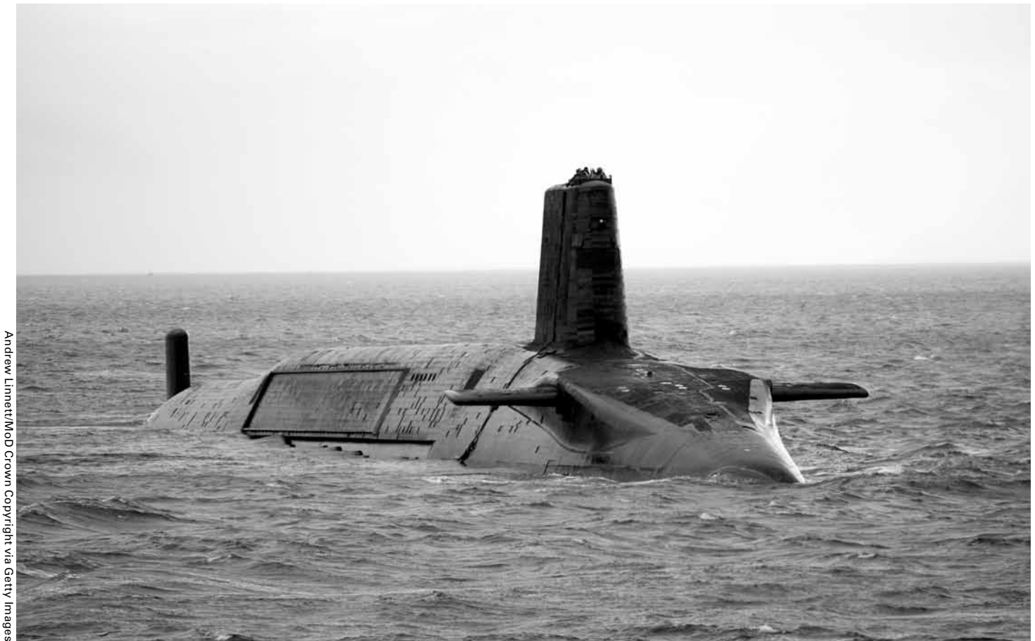
The HMS Vigilant, shown off the coast of Scotland in 2012, is one of four UK Vanguard-class SSBNs, whose nuclear propulsion reactors run on weapons-grade uranium. The Royal Navy is planning to replace these submarines with the Successor-class, powered by a new reactor, starting around 2028. U.S. Ohio-class SSBNs also use weapons-grade uranium fuel and are scheduled to be replaced with the SSBN(X), starting in 2029.
