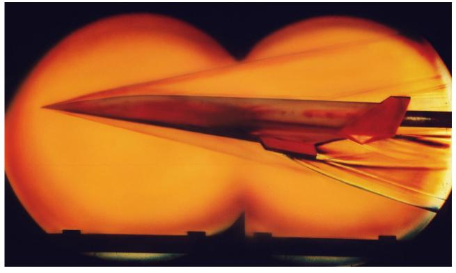
A model of a hypersonic glide vehicle is tested in a wind tunnel at NASA's Langley Research Center in Maryland on Dec. 10, 2009. (Photo by NASA's Langley Research Center)
