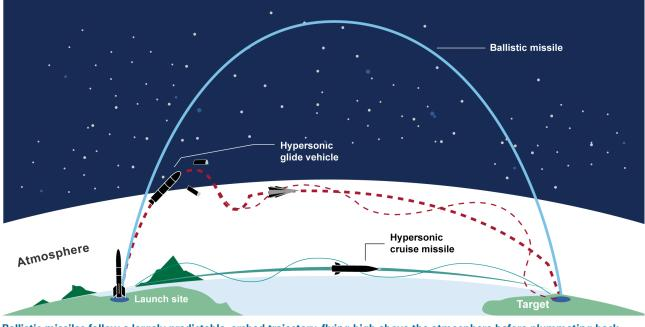
Ballistic missiles follow a largely predictable, arched trajectory, flying high above the atmosphere before plummeting back towards Earth. Hypersonic glide vehicles and cruise missiles fly at lower altitudes within the atmosphere and follow different flight paths. (Illustration by United States Government Accountability Office)
