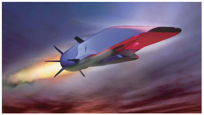
The X-51A, shown as an artist's concept, is an experimental, scramjet-powered hypersonic aircraft that achieved speeds of over Mach 5 in a 2013 test. (Graphic: U.S. Air Force)
