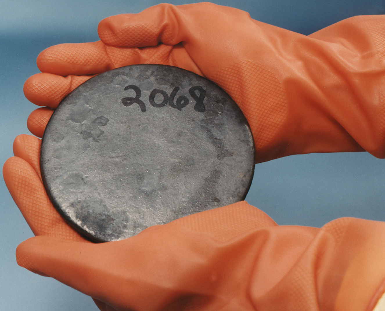
A billet of highly enriched uranium recovered from scrap processed at the Y-12 National Security Complex Plant. Original and unrotated. (Photo: U.S. Department of Energy/Public Domain)
