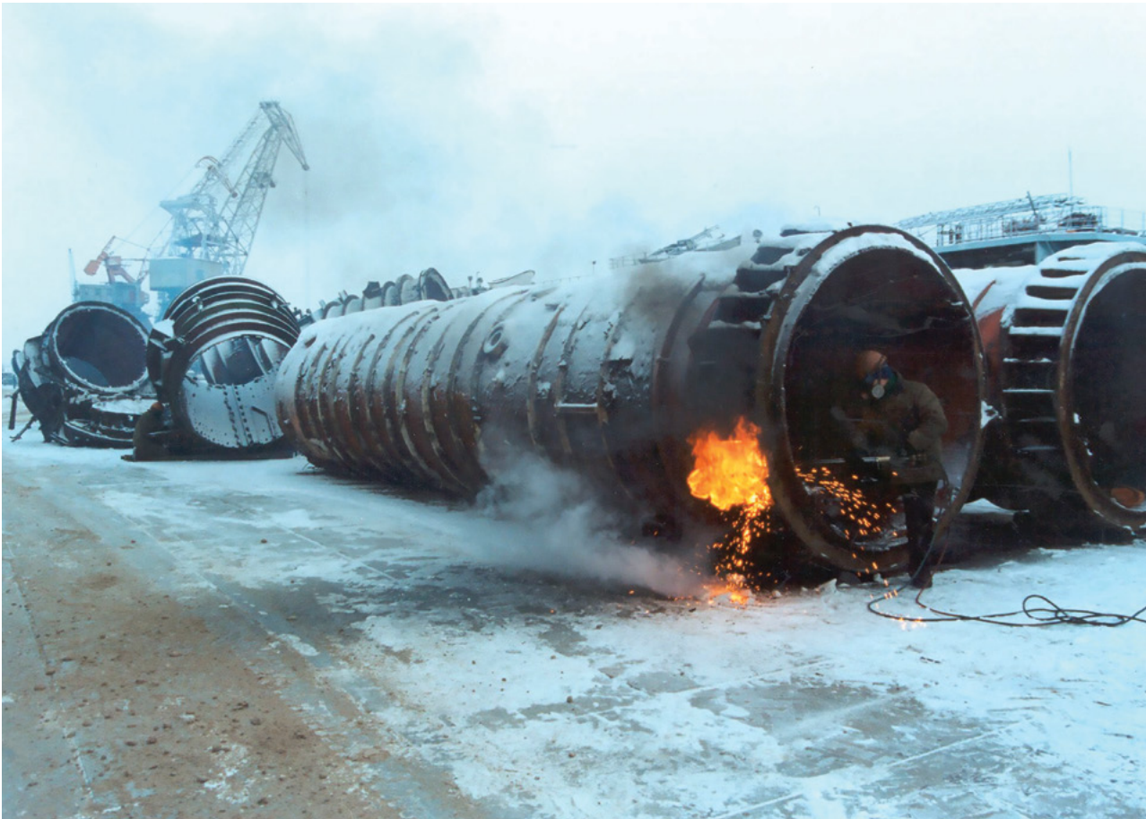
Missile launch tubes removed from a ballistic missile submarine are eliminated with equipment and services provided by the Department of Defense’s CTR program on January 29, 2010. (Photo: Defense Threat Reduction Agency)
