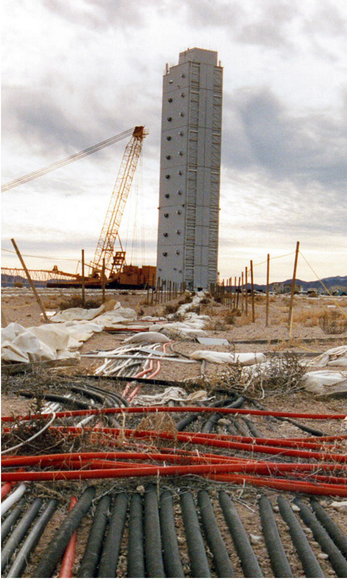
Diagnostic cables snake their way across the Nevada Test Site towards the Icecap tower, which housed the diagnostic cannister. One of three U.S. nuclear tests planned for 1993. The test was to have been in the 20-to-150-kiloton range and would have been conducted 1,557 feet underground.
